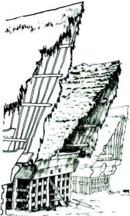
Figure 1.2c In hot and humid climates such as in Sumatra, Indonesia, native buildings are often raised on stilts and have high roofs with open gables to maximize natural ventilation.
